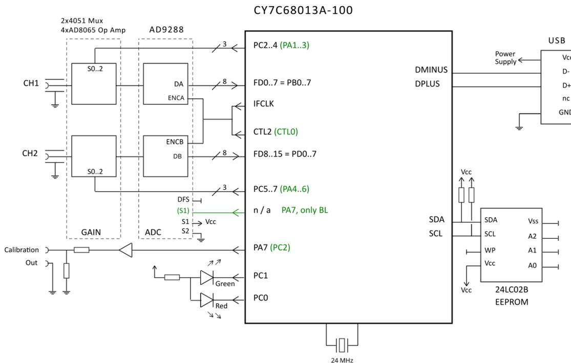
The Hantek6022 (BE & BL) backend is built around the EzUSB processor CY7C68013A that handles USB communication, ADC timing, front-end channel gain setting and also generates the calibration output signal. Hantek 6022BE and 6022BL (in scope mode) differ slightly in the use of the processor pins (**different BL pins in green**), but otherwise work identically.
