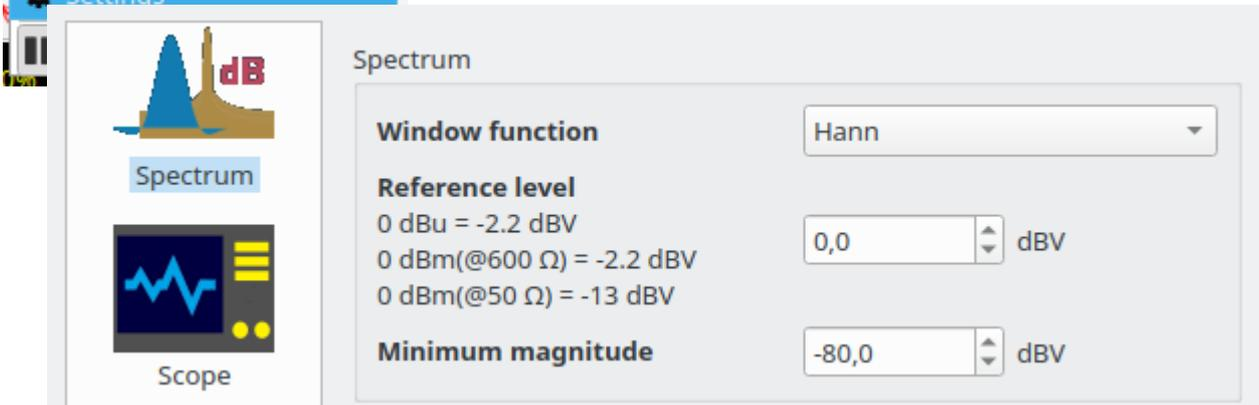
Typical window functions are Hann (raised cosine), Gauss or Flat top. The Hann window has the best frequency selectivity (narrowest bandwidth) while the Flat top window allows accurate amplitude measurements. Gauss window characteristic is in between.
