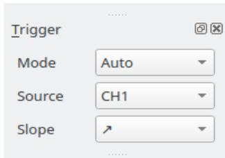
Triggering allows to display a stationary trace by fixing a rising or falling Slope of the signal of the selected Source channel to a defined position on the screen. The triggering is done in software by searching for the trigger condition in the sampled values and skipping the necessary amount of leading samples to position the trace accordingly.
