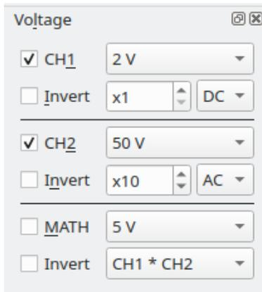
Both channels measure the voltage related to GND. **GND is directly connected also to the PC and to the main's GND so never ever connect GND of the scope to other voltages as it can destroy the scope and the PC!**
