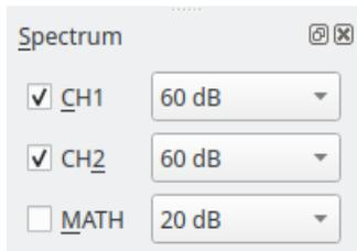
The program calculates the voltage spectrum of the three channels using the discrete FFT and displays the results if enabled. The displayed values are shown as dBV (0 dBV equals 1 V rms).
