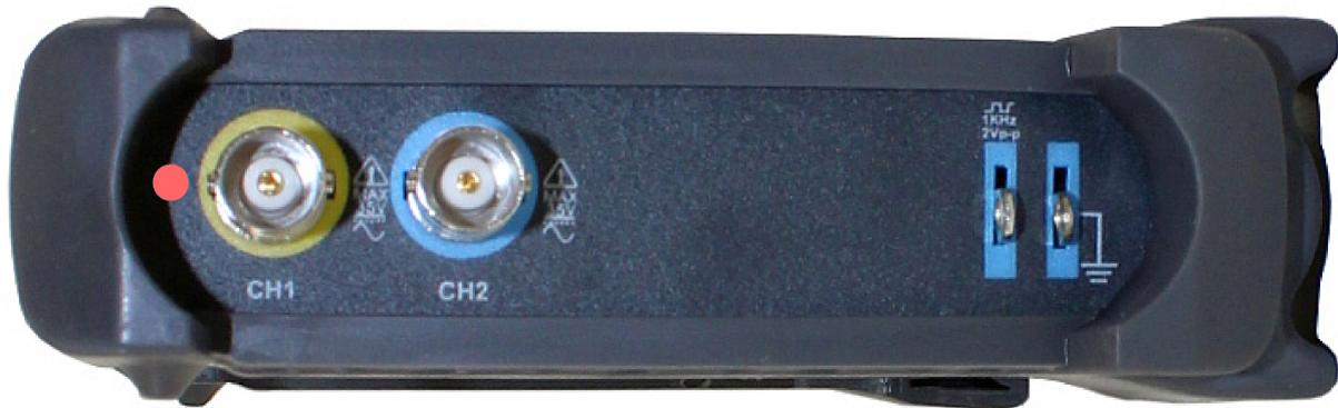
The digital storage scope Hantek6022BE (as well as the similar Hantek 6022BL) allows to measure two voltage channels CH1 (yellow) and CH2 (blue).
