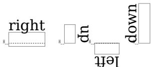
The reason that offsets are related to orientation is that we need to know in what direction the offsets have to be applied and this binding forces the user to think about it. You can also set the offsets using commands.
