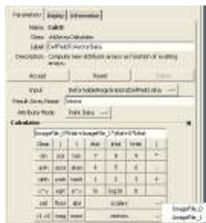
Figure 8.46: Calculators and filters may be used to compute the vector magnitude, compose vectors etc.
