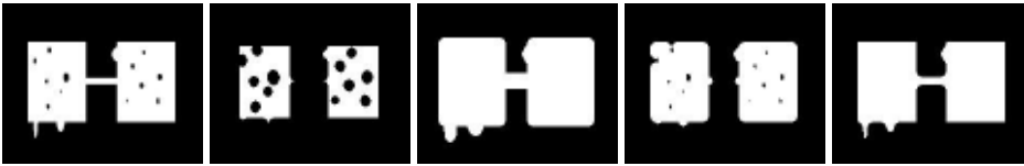
Figure 11.10: The effects of morphological operations on a binary image using a circular structuring element of size 4. From left to right are the original image, erosion, dilation, opening, and closing. The opening operation is erosion of the image followed by dilation. Closing is dilation of the image followed by erosion.
