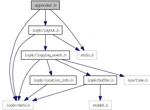
This graph shows which files directly or indirectly include this file:
